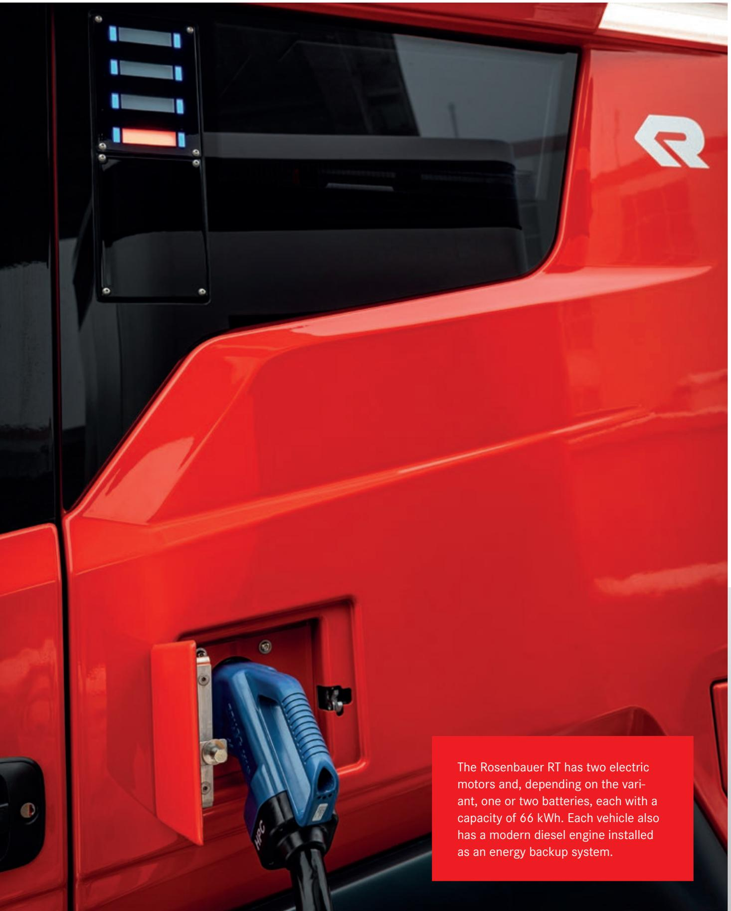
The Rosenbauer RT has two electric motors and, depending on the variant, one or two batteries, each with a capacity of 66 kWh. Each vehicle also has a modern diesel engine installed as an energy backup system.
