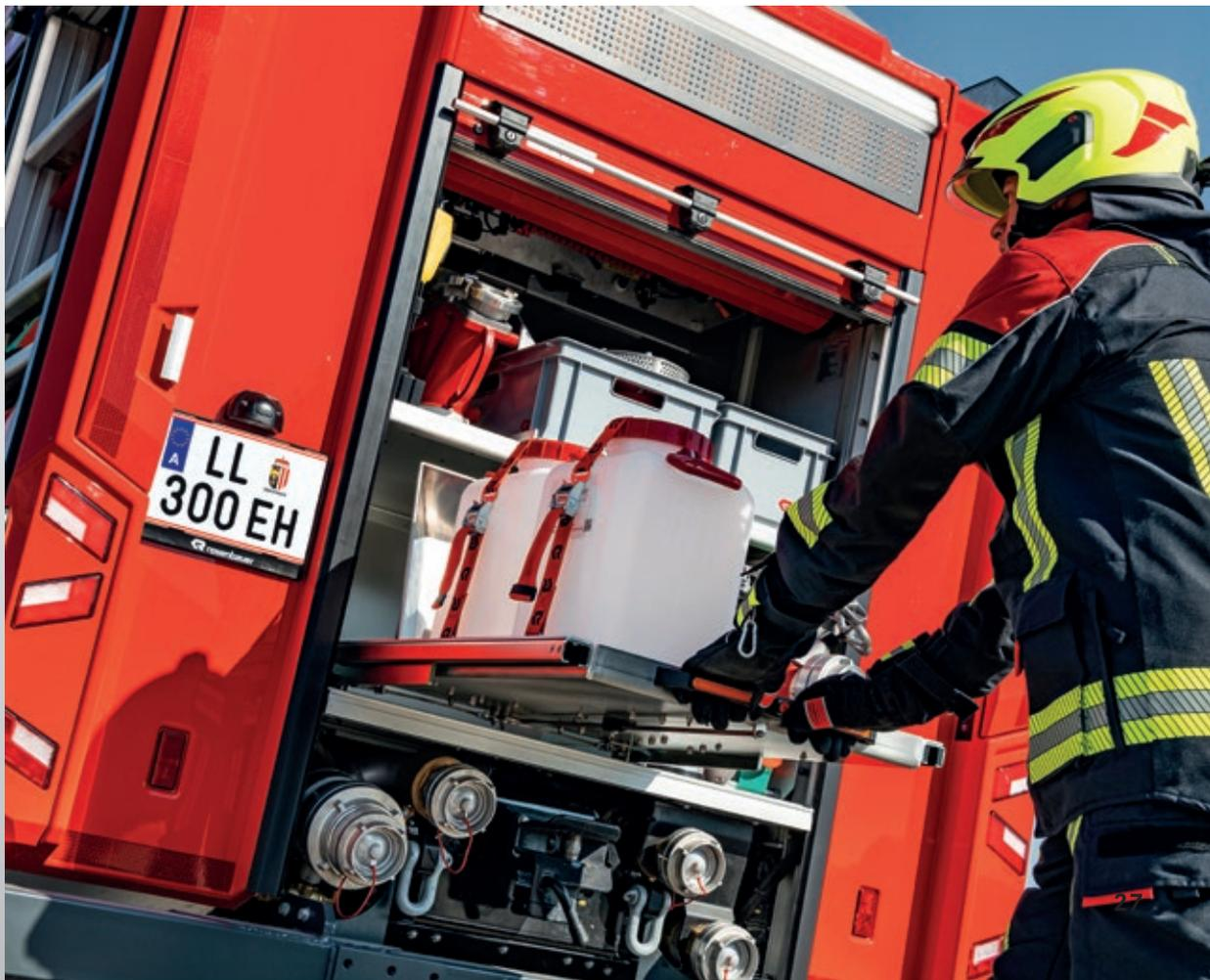
*Additional loading space at the rear thanks to the pump unit being moved forward.*
