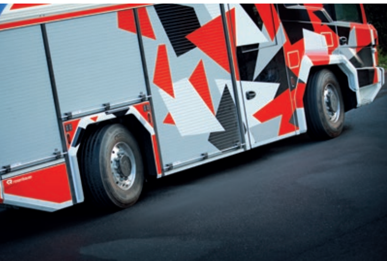
Parallel positioning of the wheels on both axles for maneuvers in confined spaces.
