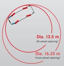
\* Turning circle diameter +/- 0.5 m – with 4,100 mm wheelbase
