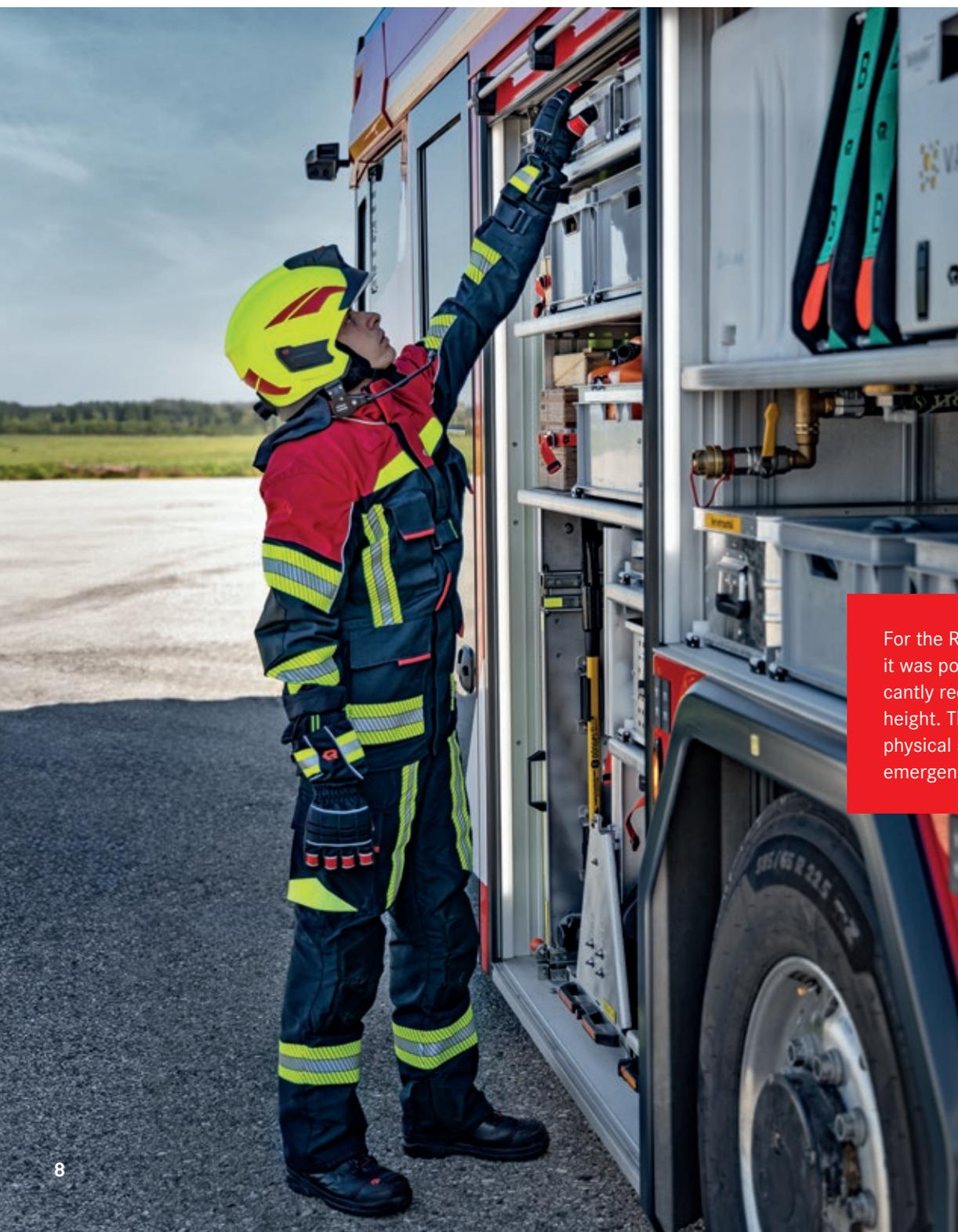
For the RT product line, it was possible to significantly reduce the removal height. This reduces the physical strain on the emergency crews.
