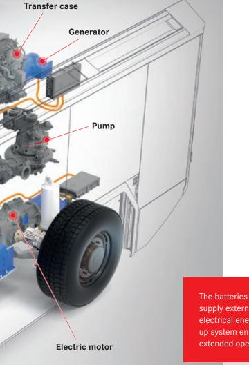
Thanks to its rechargeable batteries, the RT functions as its own power generator for equipment and auxiliary devices. And all of this without any local emissions. To ensure an uninterrupted supply of power even during extended deployments, the vehicle has a second power plant: the energy backup system.
