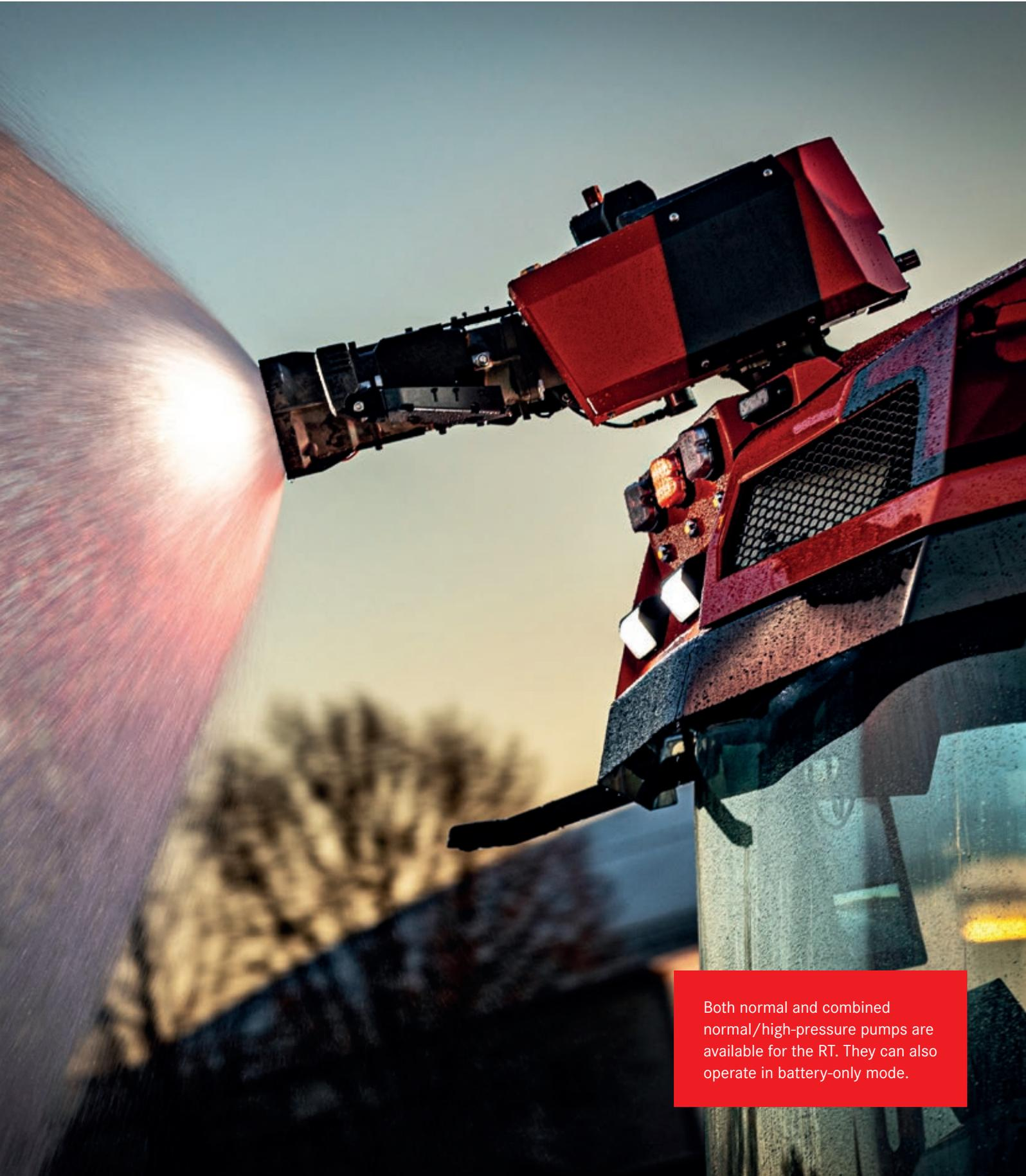
Both normal and combined normal/high-pressure pumps are available for the RT. They can also operate in battery-only mode.
