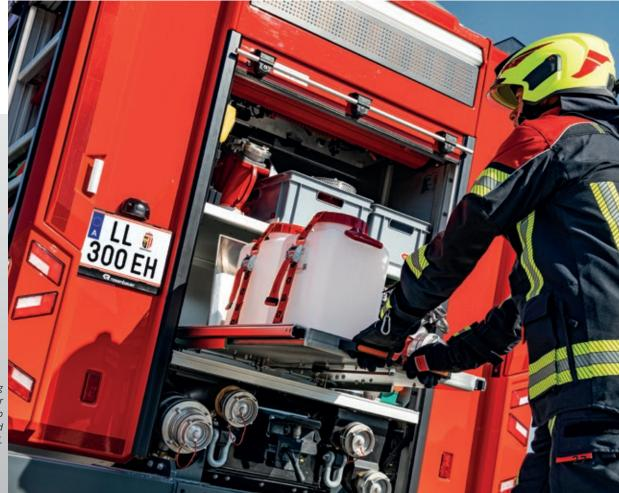
Additional loading space at the rear thanks to the pump unit being moved forward.
